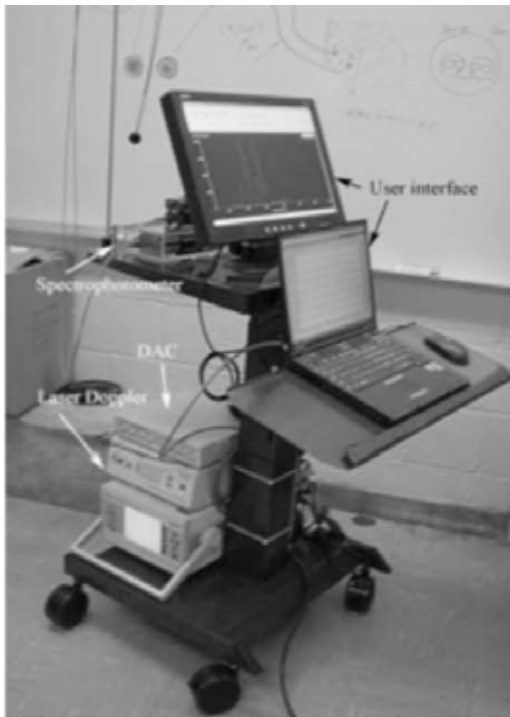
Figure 1. The clinical monitoring system, consisted of a laser Doppler unit, a spectrophotometer system, DAC board connected to pressure sensor, and a laptop computer controlling all the instrumentation.
